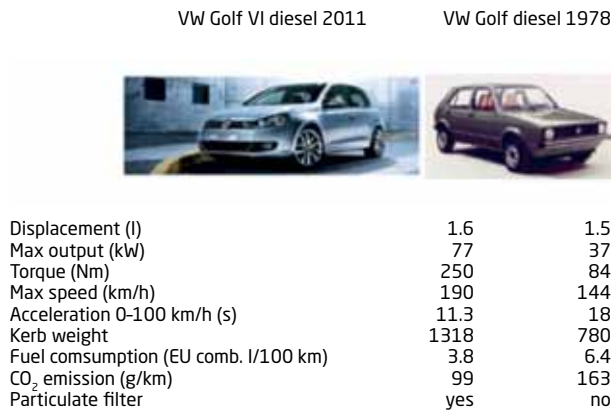
Figure 24 Comparative data for the VW Golf diesel from 1976 and 2011 [45].
