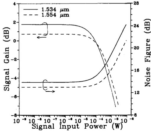
Fig. 2. Signal gain and noise figure versus the signal input power for two signal wavelengths, 1.534  $\mu\text{m}$  (solid) and 1.554  $\mu\text{m}$  (dashed). Both are calculated with 0-dB gain for pump power of 80 mW at 0.1-mW signal power.
