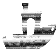
Step 2: slice CAD model
