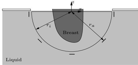
Figure 1: Schematic of the PAT Scanner. The 32 antennas are positioned in a hemispherical setup with radius  $r_a = 8$  cm and the imaging domain has a radius of  $r_i = 7.5$  cm. The breast is suspended through an aperture in the lid of the measurement tank.
