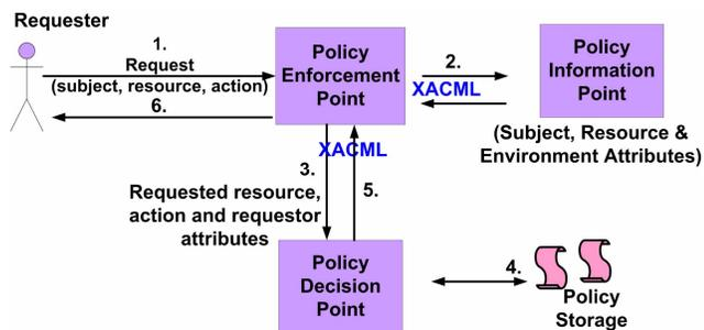
Figure 8. Policy Enforcement Architecture based on XACML flows
