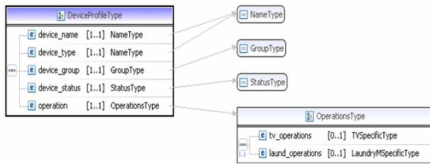
Figure 5. Example demonstrative basic ESTIA's Device Profile
