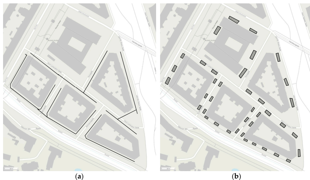
Figure 3. Distribution of NbS for Scenarios 3 and 4: (a) infiltration trench and linear garden location for Scenario 3; (b) rain garden location for Scenario 4.
