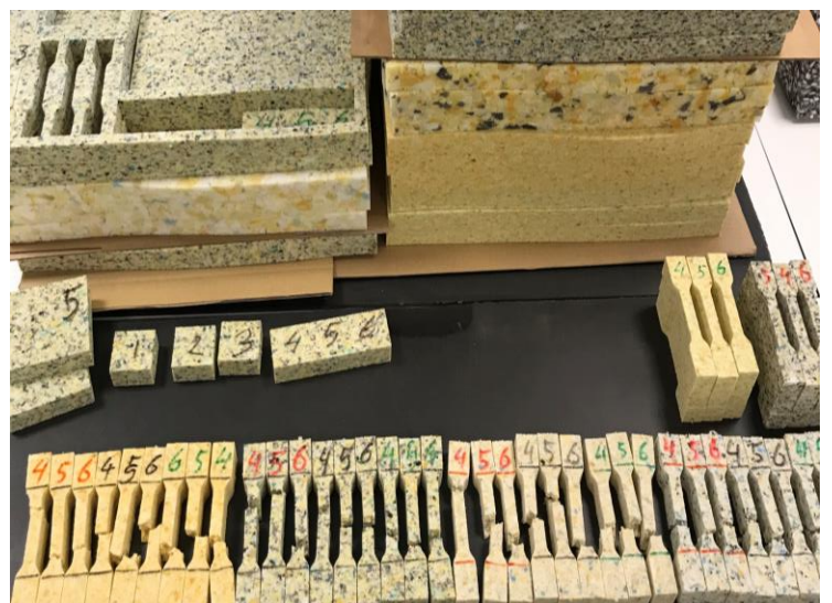
Photo: Foam samples for mechanical testing at BPI - Source: BPI 2022
