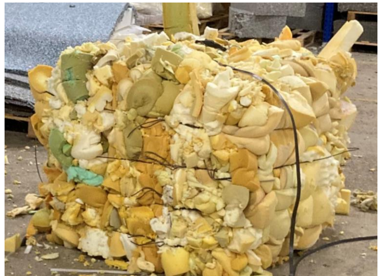
Photo: Bale of PUR foam from Danish mattresses received at BPI – Source: BPI 2022
