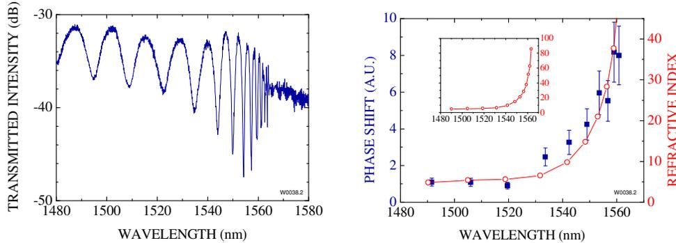
Figure 3. Left: Output power as a function of wavelength for an on-chip MZI with a 30- $\mu\text{m}$  long PCW, covered by an electrode, in one arm (device cross section as in Fig. 1[b, c]). Right: Measured phase shift (■) and effective group index (○) in the PCW.
