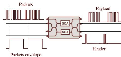
Fig. 2. Header/payload separation based on envelope detection.
