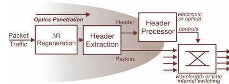
Fig. 1. Penetration path of all-optical signal processing.
