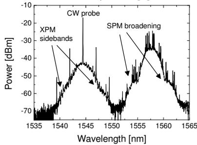
Figure 3. Output from HNLF before filtering.
