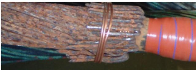
Fig. 2. Cable sample W1. The strands of the shield conductor are much closer together on this cable.
