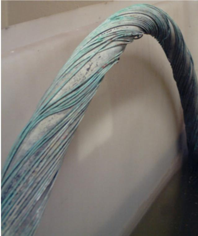
Fig. 1. Cable sample P3. Note the rather loose shield.
