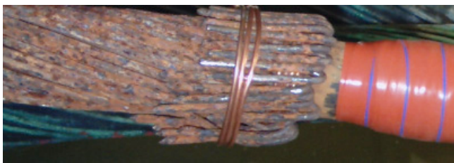
Fig. 2. Cable sample W1. The strands of the shield conductor are much closer together on this cable.
