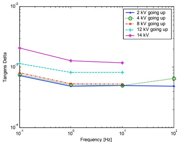
Fig. 5. Results from cable P1, a 15kV cable.
