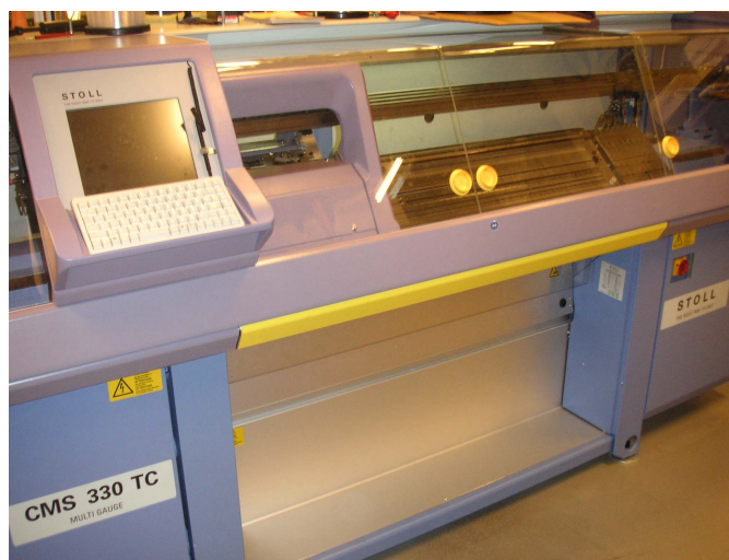
Figure 5. The flat knitting machine STOLL CMS 330 TC.
