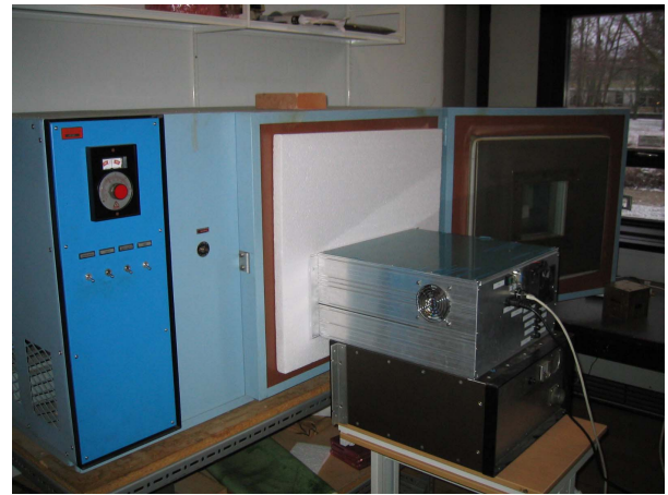
Figure 3. ACLs in test chamber for temperature characterization
