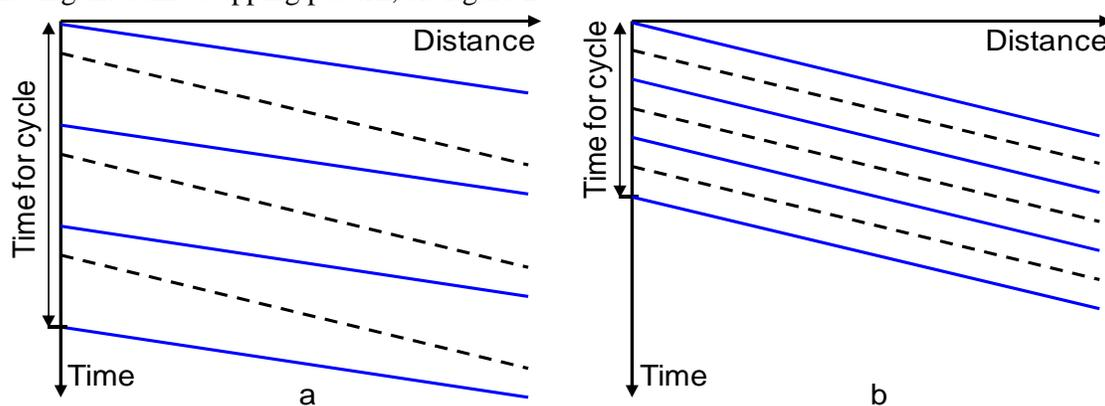
Figure 2: Heterogeneous (a) and homogeneous (b) timetable (Landex 2008).
