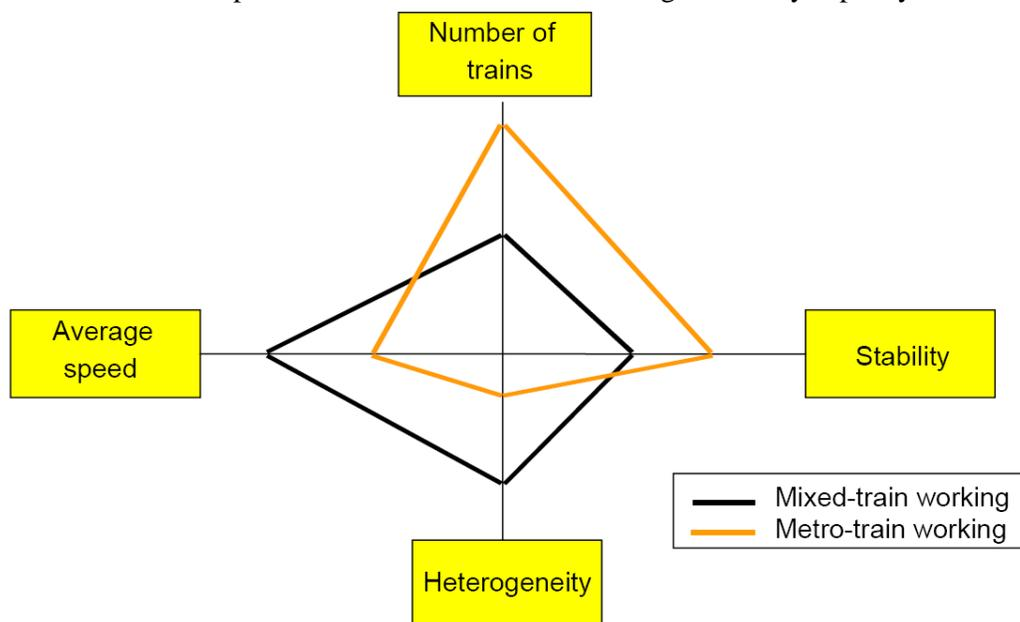
Figure 1: The balance of railway capacity (UIC 2004).
