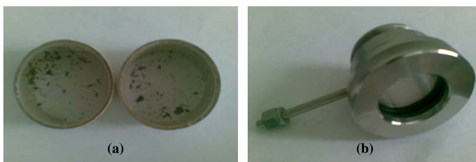
Fig 12 (a) Measurement windows contaminated with large dust particles; (b) Mounting system for observation window including a small pipe for pouring dry air.
