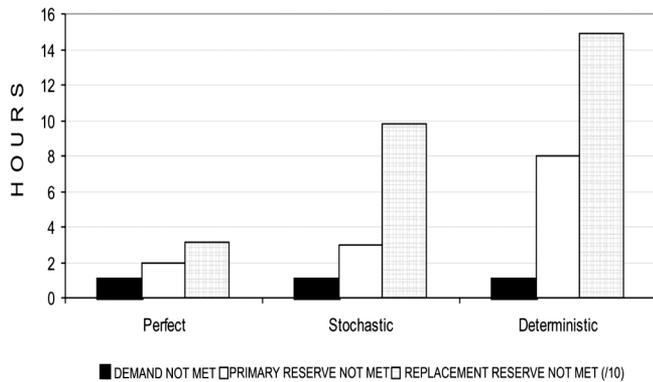
Fig. 7. Number of hours demand and reserve requirements not met over simulated year for different optimization modes, 1-h rolling. Note replacement reserve is divided by 10.
