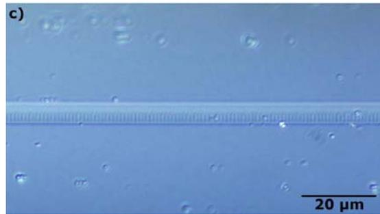
*Fig. 2: A grating written with pulse energy above threshold for damage, imaged in DIC mode (a) and in brightfield mode (b); and a DIC image of a grating written below the damage threshold, in which the laser-induced refractive index modifications can clearly be seen (c).*
