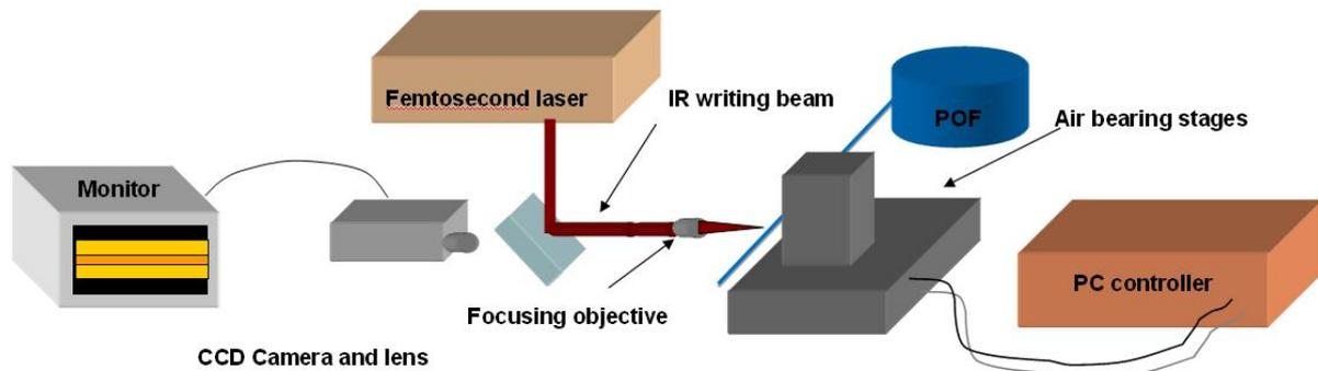
*Fig. 1: Experimental grating writing setup used*
