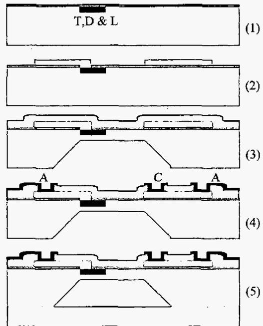
Figure 5: Chip fabrication sequence. (1) Sensors (T,D & L) are ion implanted. (2)  $\text{TiSi}_2$  wiring is formed. (3)  $\text{Si}_3\text{N}_4$  coating is applied and a membrane etched out. (4) Two metallizations form electrodes (C) and contact areas (A). (5) A Pyrex wafer is anodic bonded to the backside.
