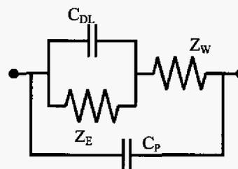
Figure 8: Conductance cell equivalent circuit. The electrolysis impedance  $Z_E$  is much higher than the water impedance  $Z_W$ . The double layer capacitance  $C_{DL}$  is higher than the parasitic capacitance  $C_P$ .
