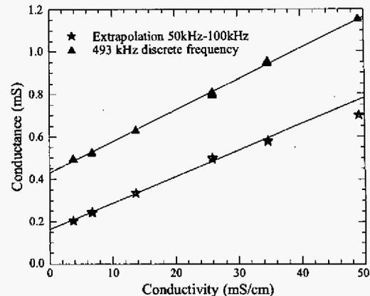
Figure 11: Measured cell conductance as a function of conductivity measured with a Radiometer CDC749 probe. Good linearity is found at a single frequency measurement ( $\blacktriangle$ ) as well as by extrapolating to infinite frequency ( $\star$ ).
