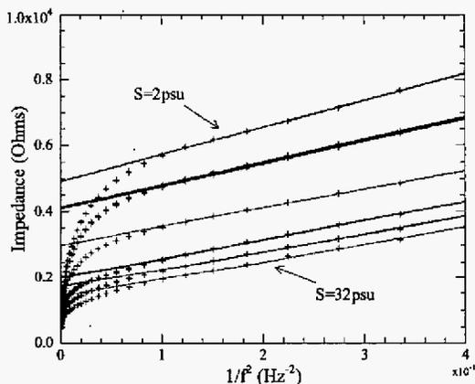
Figure 10: Measured cell impedance as a function of  $1/f^2$  at 6 different salinities (2, 4, 8, 16, 24 and 32psu). For each salinity value approx 10 measurements are super-imposed. Extrapolation to infinite frequency eliminates the double layer contribution.
