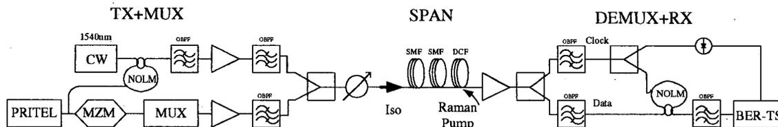
Fig. 1. Experimental set-up, OBPF: optical bandpass filter
