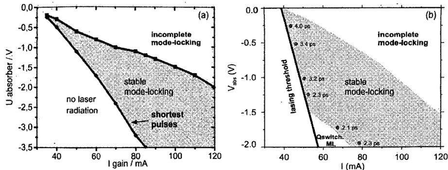
Fig. 1. Experimental (a) and simulated (b) operation regimes of a 10 GHz ECMLL composed by  $50 \mu\text{m}$  absorber,  $560 \mu\text{m}$  SOA and  $20 \mu\text{m}$  transition region. The numbers annotated in (b) correspond to the uncompressed pulsewidths.
