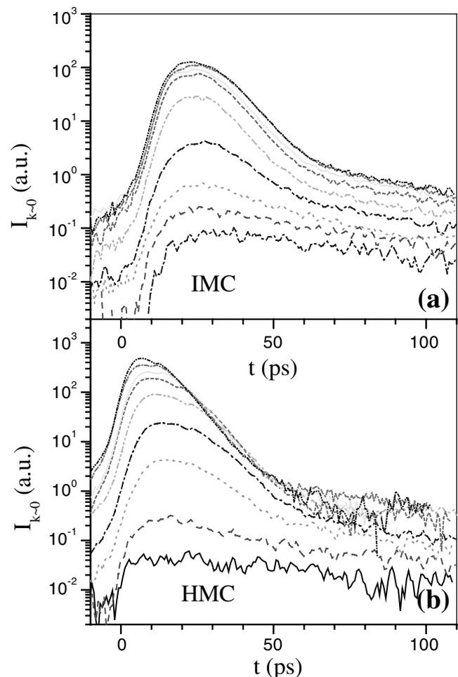
FIG. 2. Time-resolved emission for increasing excitation density ( $n_{\text{exc}}$ ) for (a) the IMC, with  $n_{\text{exc}} = (1.2, 2.0, 6.0, 12, 20, 60, 90, 120, 150) \times 10^8 \text{ cm}^{-2}$ , and (b) the HMC, with  $n_{\text{exc}} = (4.6, 9.2, 18, 36, 72, 110, 140, 180, 230) \times 10^8 \text{ cm}^{-2}$ .
