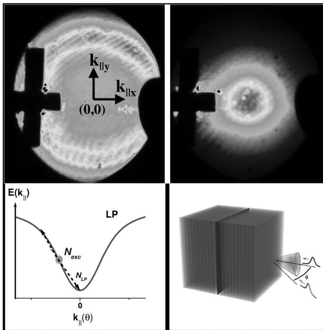
FIG. 1. The far-field emission change from a Rayleigh ring at low power ( $\sim 50 \mu\text{W}$ , upper left) to strong emission close to  $k \sim 0$  at higher power ( $> 200 \mu\text{W}$ , upper right) following angle-resonant excitation in HMC. Notice the mirror and the block for the specular pump reflection. The excitation condition on the lower-polariton branch is sketched below to the left. Below to the right is shown the experimental configuration.
