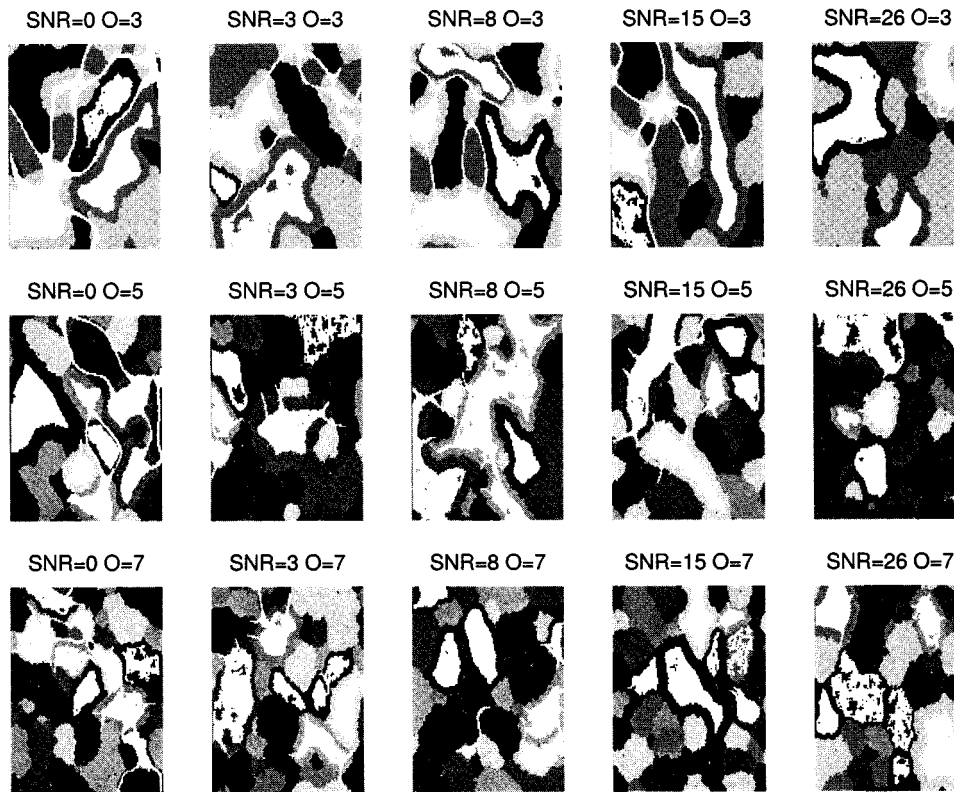
Fig. 5. The grown regions (in white) generated using the initial training sets delineated in Fig. 4 overlaid with the real thematic maps of the synthetic images shown in Fig. 3.
