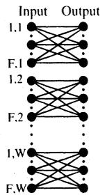
Fig. 1: Illustrates how limited wavelength conversion corresponds to multiple fibres.  $F$  fibres and  $W$  wavelengths on each fibre are shown. The number  $f,w$  to the left corresponds to the fibre and wavelength number.
