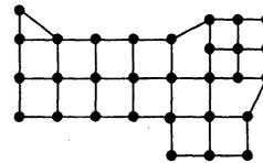
Fig.2: The NSF network, 30 nodes and 47 links.
