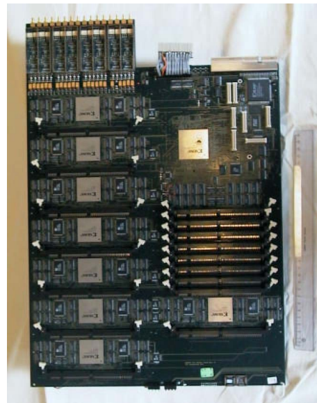
Figure 6: The receiver board layout without RAM modules to reveal the processing electronics. The board size is 53 cm by 36.5 cm.
