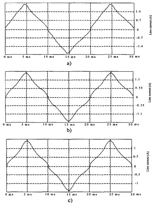
Figure 8. Input current for prototype 2 of the Modified SEPIC converter with constant peak-current control. a)  $V_{ac}=185$ ,  $\text{PF} = 0.992$ . b)  $V_{ac}=230$ ,  $\text{PF} = 0.990$ . c)  $V_{ac}=270$ ,  $\text{PF} = 0.986$
