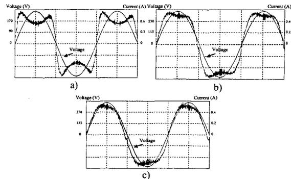
Fig. 7. Input-current of the Modified SEPIC converter with fast output regulation a)  $V_{in} = 185\text{Vac}$ ,  $\text{PF}=0.89$ . b)  $V_{in} = 230\text{Vac}$ ,  $\text{PF}=0.97$ . c)  $V_{in} = 270\text{Vac}$ ,  $\text{PF}=0.98$ .
