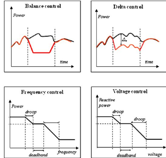
Fig. 2. Different control functions in modern wind farms.
