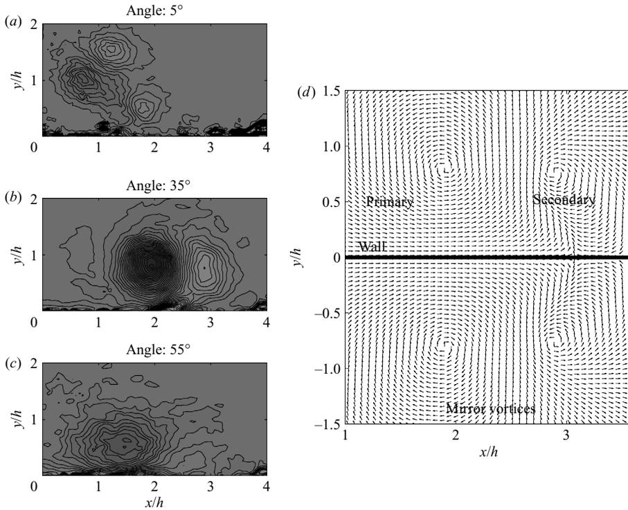
FIGURE 3. Iso-contour maps of axial vorticity for device angles (a)  $\beta = 5^\circ$ , (b)  $\beta = 35^\circ$  and (c)  $\beta = 55^\circ$ . In (d) a sketch showing a sample velocity distribution of the primary and secondary (upper half) and mirror vortices (lower half) is presented. The wall is illustrated by a thick line at  $y/h = 0$ .
