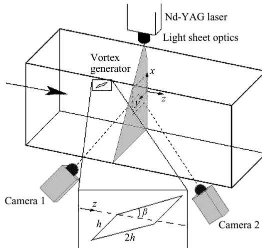
FIGURE 2. Schematic illustration of the experimental set-up and device geometry. The large arrow to the left indicates the main flow direction and  $\beta$  the device angle. The measurement plane in the laser sheet has been indicated by dashed lines.
