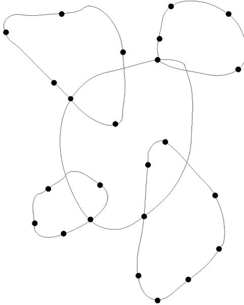
Figure 1: Two-layered ring network. A set of 23 nodes are connected through a two-layer hierarchical network with the federal ring connecting the metro rings.
