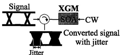
Fig. 1: Jitter arising from counter-propagation in an XGM converter.
