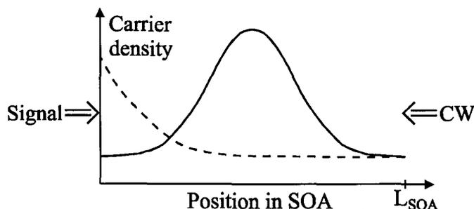
Fig. 2: Carrier density distributions in the XGM-SOA for a fixed CW power with an equal (—) and a higher (- -) signal power level.
