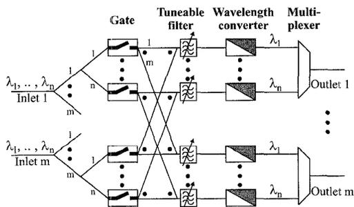
gates and combiners. The gates are based on SOAs offering a high on/off ratio (40-50 dB) and a high gain (30 dB). After the space switching stage tuneable filters are used to select the desired wavelength channel. Finally, interferometric wavelength converters with fixed output wavelengths allow for multiplexing the selected channels.
