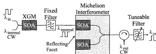
As the XGM converter is followed by another converter capable of conversion to longer wavelengths these drawbacks will not influence the performance of the dual-stage converter. This is assured by choosing the internal wavelength shorter than the shortest of the network wavelengths. After the XGM converter the dual-stage converter exploits the excellent chirp characteristics of the XPM converter together with its capability to regenerate the extinction ratio.
