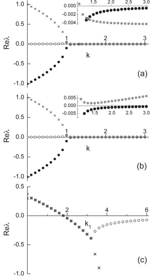
Figure 1: Real parts of the largest eigenvalues versus the control gain  $k_1$  for  $b = 0.01$ . (a) from Eq. (13) with  $\omega_1 = 0.001$ , (b) from Eq. (14) with  $\omega_1 = 0.001$ ,  $\tau = 0.007$ , (c) from Eq. (26) with  $\omega_1 = 0.3$ ,  $\tau = 0.007$ ,  $\omega_2 = 7$ ,  $k_2 = 17$ . The set of the control parameters,  $\omega_1$ ,  $\omega_2$ , and  $k_2$  is somewhat arbitrary and empirical.
