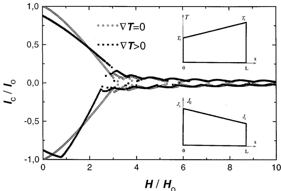
FIG. 6. Numerically calculated dependencies  $I_c(H)$  for a long Josephson junction (i) without a temperature gradient (open circles) and (ii) with a temperature gradient ( $\nabla T=0.02$ ) (solid squares). In the inset spatial distributions of the temperature and the critical current densities are shown schematically.
