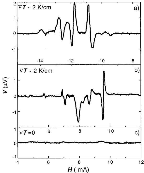
FIG. 13. Experimental dependencies  $V(H)$  for the Nb-NbO<sub>x</sub>-Pb junction for zero applied current and for different directions of the magnetic field. In (c) there is no temperature gradient and in (a) and (b) a temperature gradient of about 2 K/cm is applied while the mean temperature of the junction was about 5.5 K. It is seen that application of a temperature gradient causes generation of ZCFFS's.
