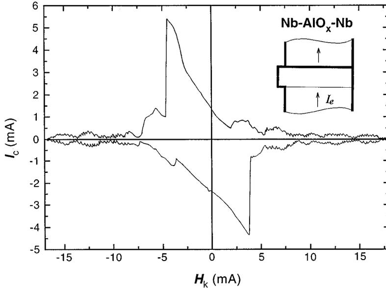
FIG. 7. Experimental dependence  $I_c(H)$  for a Nb-AIO<sub>x</sub>-Nb junction with  $L = 30\lambda_J$  at  $T = 4.2$  K. In the inset the junction geometry is shown schematically. Two periods in magnetic field are well defined, the larger period being about ten times the smaller one.
