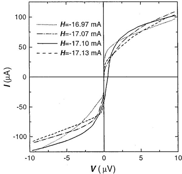
FIG. 9. Experimental  $I$ - $V$  curves of the Nb-AlO<sub>x</sub>-Nb junction in larger scale at  $T=4.2$  K and for different magnetic fields near the field at which the critical current in one of the directions vanishes. A zero crossing flux flow step is observed at  $H=-17.10$  mA (solid curve).
