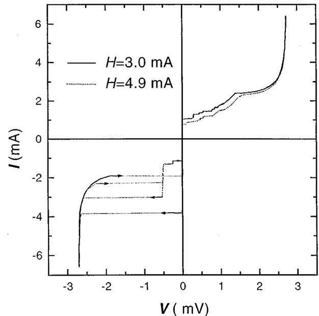
FIG. 8. Experimental  $I$ - $V$  curves for the same Nb-AIO<sub>x</sub>-Nb junction at two different magnetic fields and  $T = 4.2$  K. Asymmetry of FFS's for positive and negative directions of the bias current is clearly visible.
