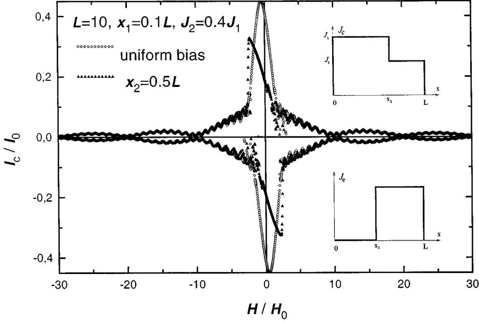
FIG. 3. Numerically calculated  $I_c(H)$  dependencies for a steplike critical current distribution with  $J_{c2} = 0.4J_{c1}$  and  $x_1 = 0.1L$  for uniform bias (open circles) and step-like bias current distribution (solid triangles)  $J_{e1}(x) = 0 \{0 < x < x_2\}$ ,  $J_{e2}\{x_2 < x < L\}$ ,  $x_2 = 0.5$ . Spatial distributions of the critical and bias currents are shown schematically in the insets.
