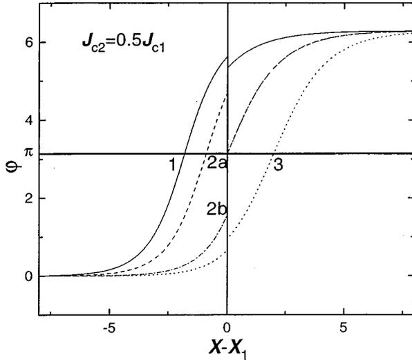
FIG. 2. Spatial dependence of the phase difference for a single fluxon in a junction with a steplike critical current distribution  $J_{c2} = 0.5J_{c1}$ , for different positions of the fluxon center: (i) to the left of the boundary, curve 1, (ii) at the boundary, curves 2a and 2b, and (iii) to the right of the boundary, curve 3. It is seen that a switching from curve 2a to curve 2b occurs when the fluxon crosses the boundary  $x = x_1$ .
