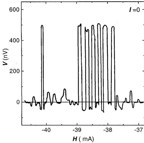
FIG. 11. The same as in Fig. 10(b) for different field range. It is seen that in addition to small oscillating ZCFFS's, large positive ZCFFS's with  $V \sim 0.5 \mu\text{V}$  are present corresponding to fluxon motion in the direction of smaller critical current.
