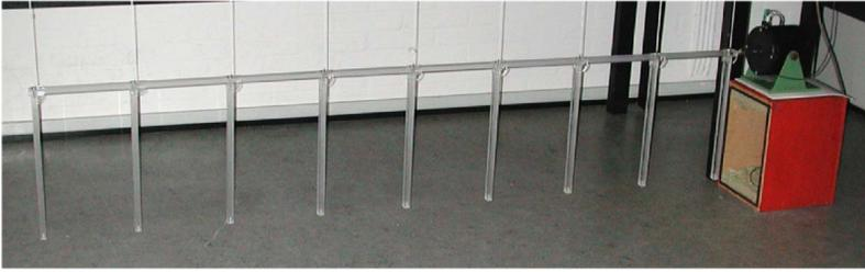
FIG. 7. Experimental arrangement. Point force excitation in longitudinal direction at junction 0.
