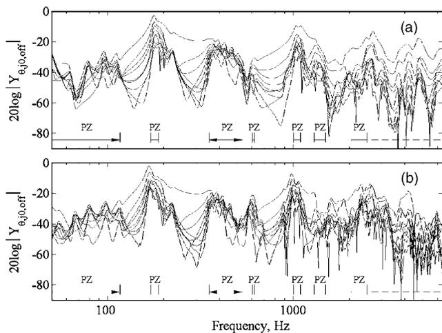
FIG. 11. Junction rotational mobilities  $Y_{\theta_j,0,off} = \dot{\theta}_j / F_{0,off}$ , for  $j=0-8$ , of finite periodic structure with eight elements; the system is driven by an offset harmonic point force  $F_{0,off}$  acting on the first transverse beam at 183 mm below junction 0. (a) Numerical predictions using Eq. (42), and (b) measurements.
