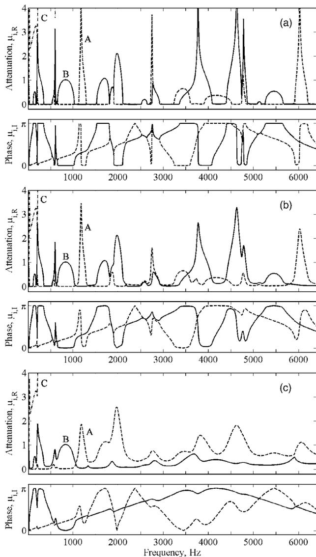
FIG. 2. Frequency variation of the real and imaginary parts of the propagation constants  $\mu_i = \mu_{i,R} + j\mu_{i,I}$  for the three wave-types: (---) flexural-longitudinal wave A; (—) flexural-longitudinal wave B; (-·-) predominantly flexural near-field C. Damping loss factors: (a)  $\eta=0.001$ ; (b)  $\eta=0.01$ ; (c)  $\eta=0.056$ .
