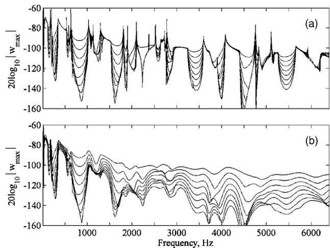
FIG. 4. Maximum transverse displacements  $w_{max}$  in column component of the first eight elements of semi-infinite periodic structure. Excitation by a harmonic point moment of unit amplitude. Damping loss factors: (a)  $\eta=0.001$ ; (b)  $\eta=0.056$ .
