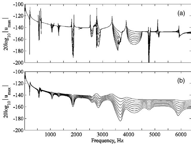
FIG. 5. Maximum longitudinal displacements  $u_{\max}$  in column component of the first eight elements of semi-infinite periodic structure. Excitation by a harmonic longitudinal point force of unit amplitude. Damping loss factors: (a)  $\eta=0.001$ ; (b)  $\eta=0.056$ .
