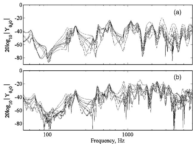
FIG. 10. Junction rotational mobilities  $Y_{\theta,j0} = \dot{\theta}_j / F_0$ , for  $j=0-8$ , of finite periodic structure with eight elements; the system is driven at junction 0 by a longitudinal point force. (a) Numerical predictions using Eq. (42), and (b) measurements.
