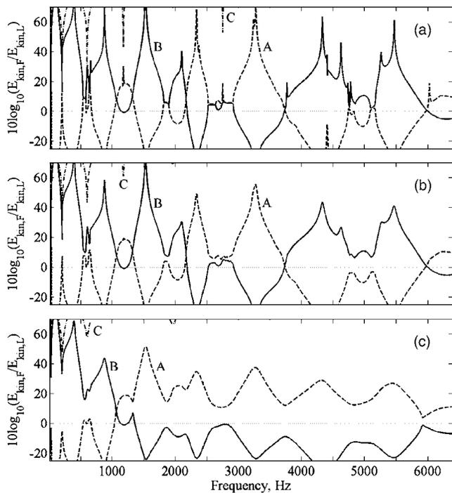
FIG. 3. Energy ratios  $E_{kin,F}/E_{kin,L}$  for the three wave-types: (---) flexural-longitudinal wave A; (—) flexural-longitudinal wave B; (-·-) predominantly flexural near-field C. Damping loss factors: (a)  $\eta=0.001$ ; (b)  $\eta=0.01$ ; (c)  $\eta=0.056$ .
