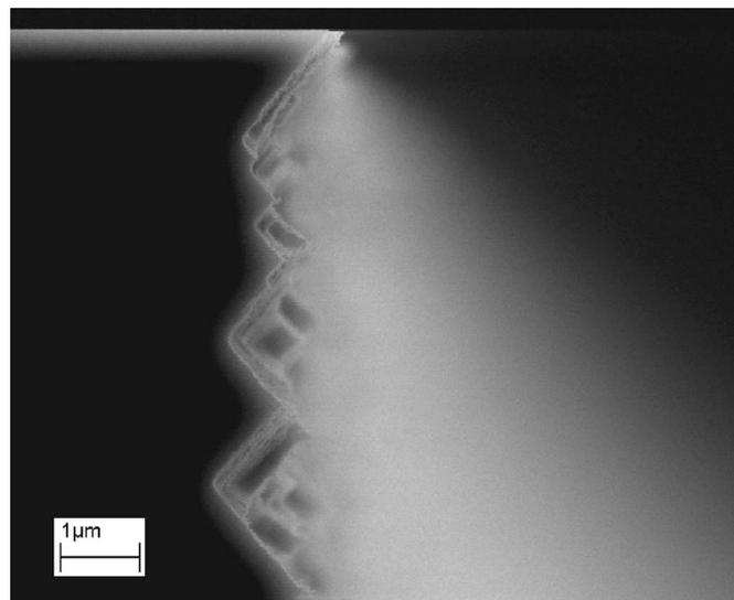
**Figure 7.** SEM closeup of the sidewall roughness in highly rough etching process, recipe M. The facets of the sidewall roughness have angles in good agreement with the expected angles of {111} planes.
