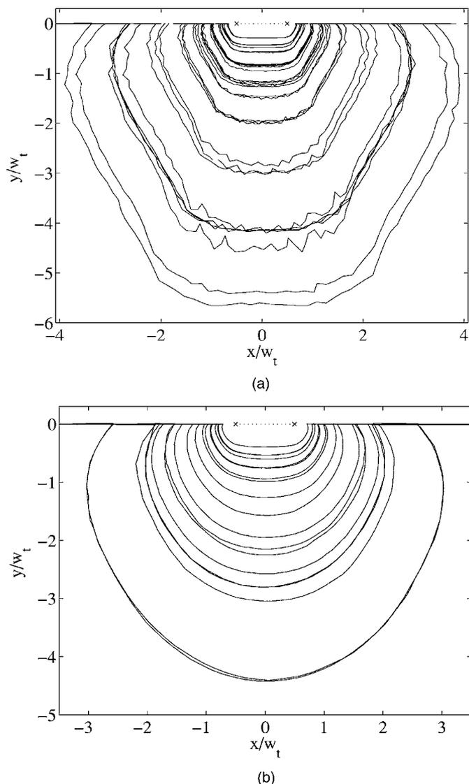
**Figure 3.** Digitized etched profiles normalized to the mask window width,  $w_t$ , for etching processes with an ICP power of 3000 W, window width  $w_i = 7\text{--}180\ \mu\text{m}$  and the pressure  $p = 70\ \text{mTorr}$  (top) or  $p = 10\ \text{mTorr}$  (bottom).
