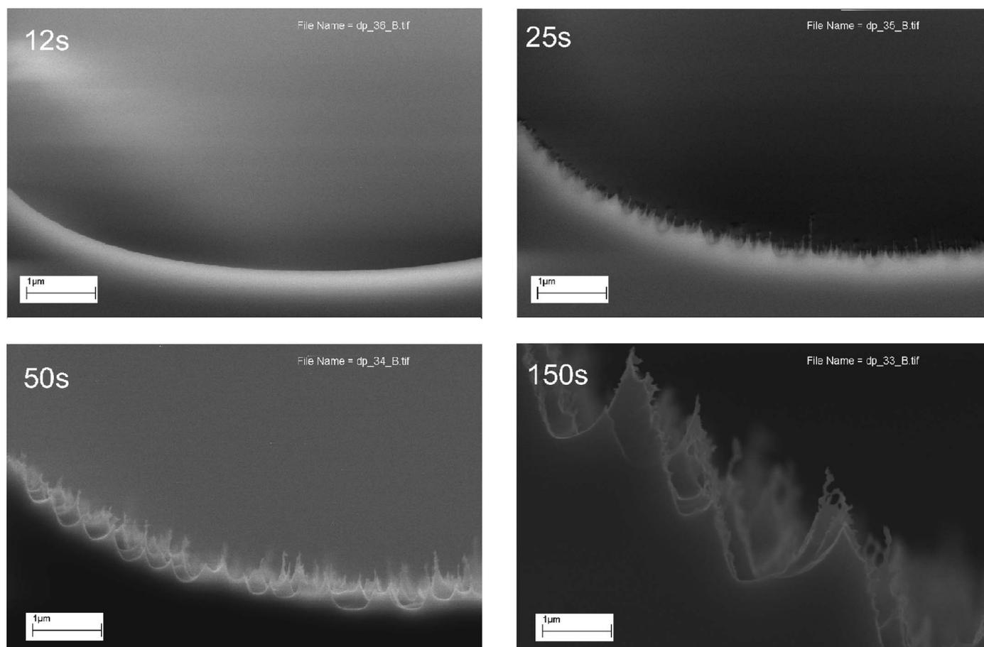
**Figure 6.** SEM images of the temporal evolution of the roughness for etching processes using recipe M with a mask width of 7 μm at elapsed etch times of 12, 25, 50, and 150 s. Note that the magnification is the same in all images.
