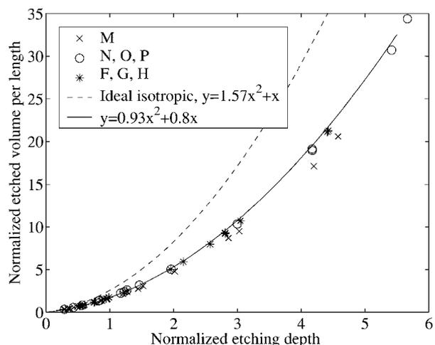
**Figure 10.** The normalized etched volume per length,  $V_{\text{etch}}/(Lw_t^2)$ , as a function of the normalized etched depth,  $h_{\text{bot}}/w_t$ .
