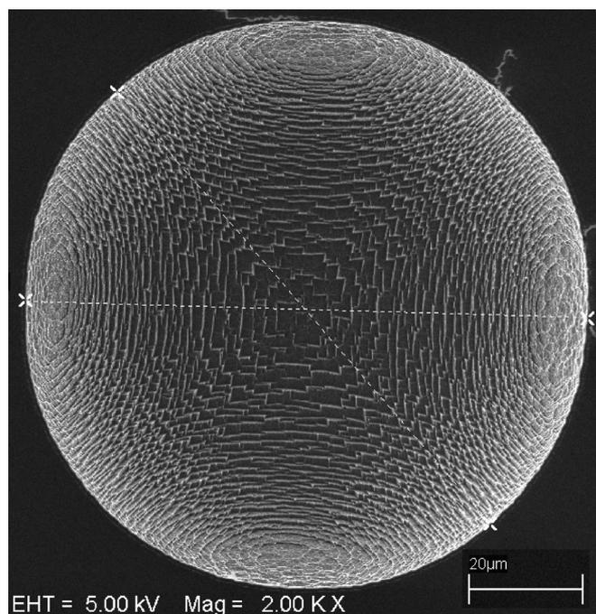
**Figure 8.** SEM image showing a top view of an etched circular cavity with roughness type IV (etching recipe comparable to recipe I). The crystal-orientation-dependent roughness in the cavity is related to the {111} planes of silicon. The horizontal diameter is 98.7 μm ( $\langle 110 \rangle$  directions), and the 45° diam is 100.8 μm ( $\langle 100 \rangle$  directions); thus, the etch rate differs by only 2% in these crystal directions.
