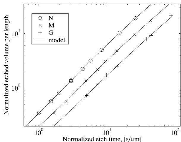
**Figure 12.** Experimental profile data and results from the etching model plotted against the normalized etching time,  $t_{\text{etch}}/w_l$ .
