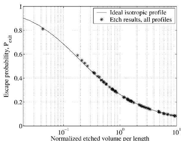
**Figure 11.** The escape probability,  $P_{\text{exit}}$ , of a radical through the mask window as a function of the normalized etched volume per length,  $V_{\text{etch}}/(Lw_l^2)$ .
