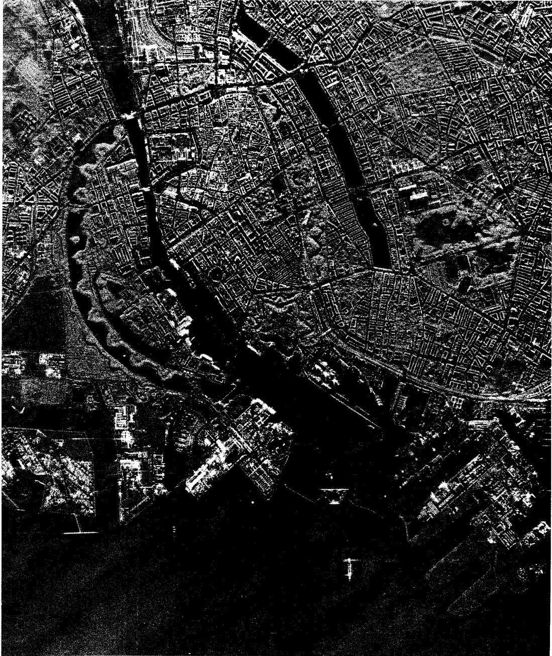
Figure 5. C-band SAR image of Copenhagen showing the city center and the harbour from 25 km distance. The image width is 6 km and the resolution is 2 by 2 meters.
