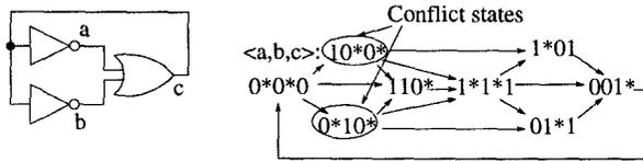
Figure 1: Speed-independent (by Muller) but not semimodular circuit.
