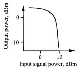
Fig. 5. Schematic of output versus input power characteristic for laser converter.
