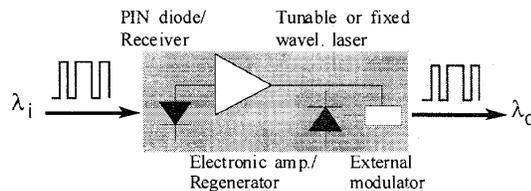
Fig. 3. Schematic of opto-electronic converter.
