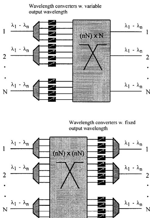
Fig. 1 Schematic of switch blocks with wavelength converters.
