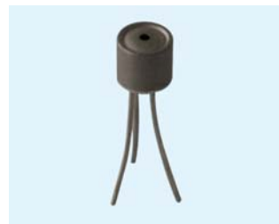
Figure 1 Microphones with a diameter of around 4 mm installed about 1 mm below the surface of the airfoil to measure high frequency surface pressure fluctuations
