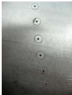
Figure 1 Microphones with a diameter of around 4 mm installed about 1 mm below the surface of the airfoil to measure high frequency surface pressure fluctuations
