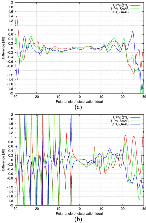
Fig. 3 Logarithmic difference between the co-polar patterns: (a)  $\phi = 0^\circ$  plane and (b)  $\phi = 90^\circ$  plane.
