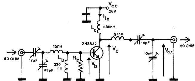
Fig. 1. 160-MHz power amplifier. Performance data: output power—13.8 W; gain—9 dB; and collector efficiency—73 percent.
