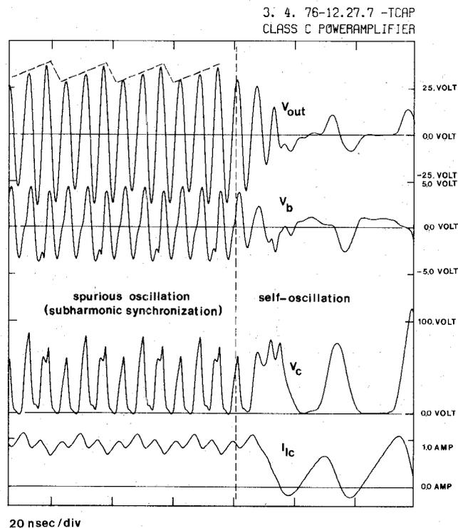
Fig. 5. Spurious oscillations in the amplifier of Fig. 1 using  $L_b = 20$  nH,  $R_b = 50 \Omega$ , and a slightly detuned output matching network which corresponds to a mismatch of  $VSWR = 2.2, -60^\circ$ . At the time given by the dashed line, the generator is turned off and the self-oscillation becomes visible.
