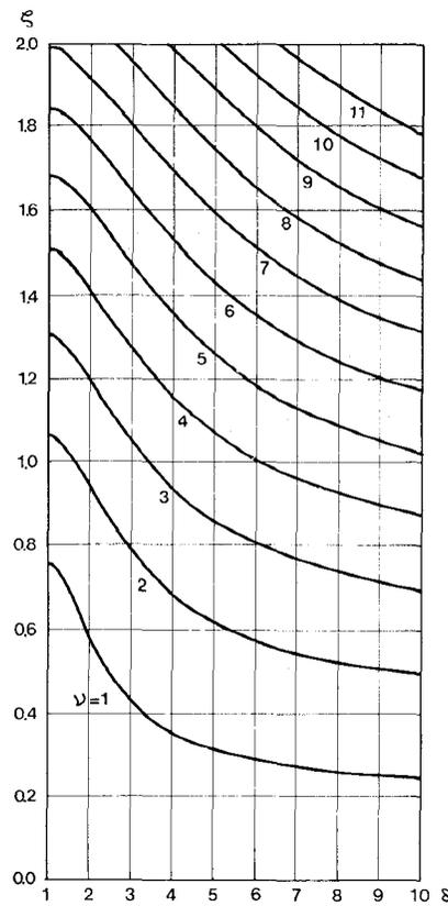
Fig. 15. Contours showing the solutions to (26) using  $\nu$  as parameter. For a given  $\nu$  the magnitudes of  $\xi$ ,  $\delta$ , which assure suppression of the self-oscillation, lie above the corresponding contour.
