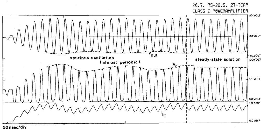
Fig. 3. Simulated response of the amplifier shown in Fig. 1 using  $R_b = 470 \Omega$  and nominal operation conditions. At the time given by the dashed line a numerical steady-state analysis is employed.
