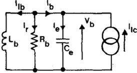
Fig. 10. Equivalent diagram for the base-emitter circuit in the cutoff period.
