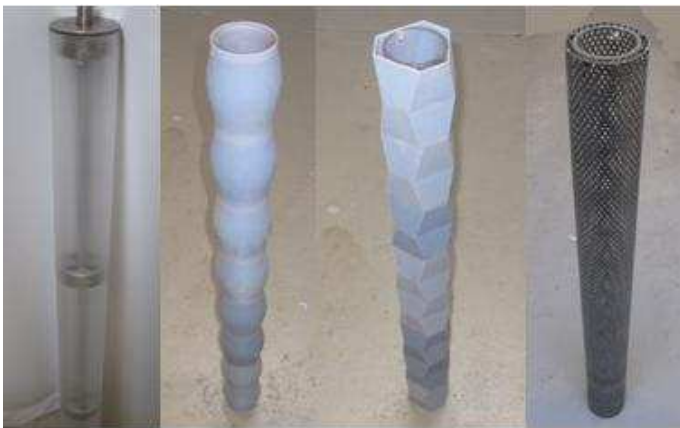
Figure 3: Section models (from right to left), plain cylinder, wavy cylinder, faceted cylinder and shrouded cylinder.
