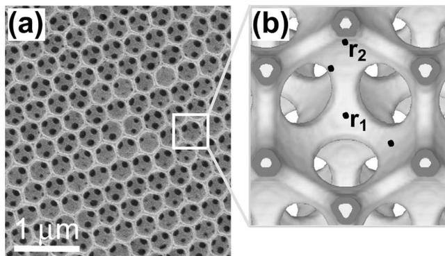
FIG. 1. (a) Electron-microscope image of the (111) surface of an inverse opal consisting of air spheres in  $\text{TiO}_2$  with lattice parameter  $a=425$  nm. (b) Schematic of quantum dots (black spots) on the internal titania-air surfaces at symmetry-inequivalent positions  $r_i$  in the crystal unit cell.
