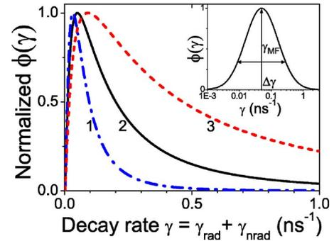
FIG. 3. (Color online) Decay-rate distributions  $\phi(\gamma)$  for the inverse opals with lattice parameters  $a=425$  nm (1),  $a=255$  nm (2), and  $a=540$  nm (3), corresponding to the data shown in Fig. 2. The inset shows  $\phi(\gamma)$  for  $a=255$  nm in the semilogarithmic scale. Clear modifications of  $\Delta\gamma$  and  $\gamma_{MF}$  with varying lattice parameter of the inverse opals are seen.
