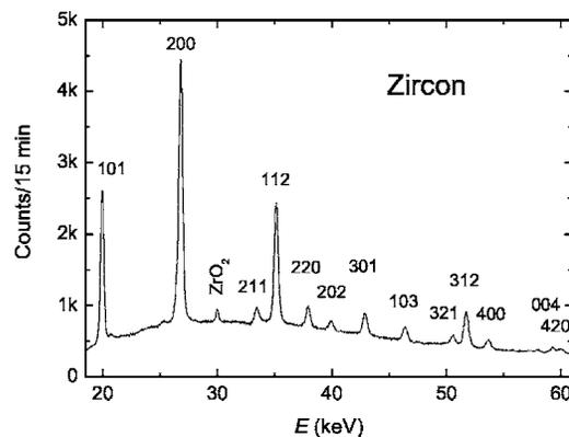
FIG. 1. Energy-dispersive x-ray diffraction spectrum of zircon at ambient pressure. The small peak at about 30 keV is due to zirconium oxide. The Bragg angle is  $\theta=4.01^\circ$ . The strong zirconium fluorescence lines (at 15.7 and 16.7 keV) are not shown.
