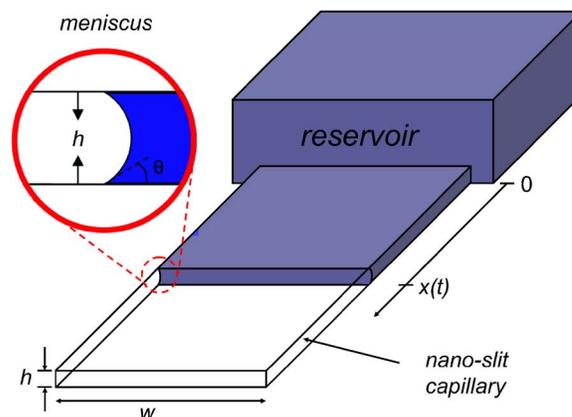
FIG. 1. (Color online) Schematic illustration of a nanoslit-capillary filling experiment. A nanoslit capillary, of height  $h \leq 300$  nm and width  $w$  several micrometers is filled with liquid from an attached reservoir by capillary action. The length of the fluid plug—the position of the liquid meniscus— $x(t)$  is recorded as function of time  $t$ .
