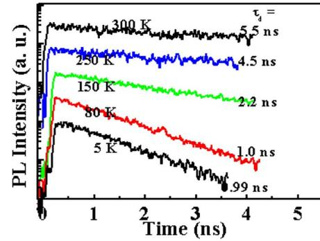
FIG. 3. (Color online) Time decay of PL detected at the peak energies at different temperatures.
