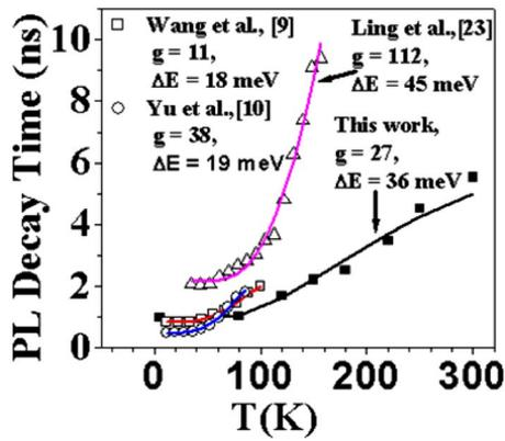
FIG. 4. (Color online) The PL decay times of InGaAs/GaAs QDs vs temperature (closed squares). Open symbols represent data from the literature. The solid lines show the fitting results. The fitting parameters are given in the figure.
