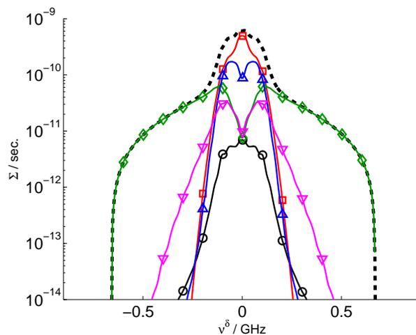
**Figure 11.** Scattering function for minority  $^3\text{He}$  ICRH; selection of near parallel velocities; scattering parameters:  $R = 6.76$  m,  $Z = 0.59$  m,  $\phi = 2^\circ$ ,  $\theta = 16^\circ$ ;  $\diamond$ -alphas,  $\triangle$ -tritons,  $\nabla$ - $^3\text{He}$ ,  $\square$ -bulk ions,  $\circ$ -electrons, ----total
