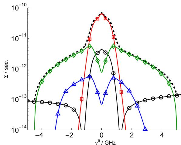
**Figure 9.** Scattering function for location in the NBI beam path; selection of near perpendicular velocities; scattering parameters:  $R = 6.12$  m,  $Z = 0.64$  m,  $\phi = 101^\circ$ ,  $\theta = 162^\circ$ ;  $\diamond$ -alphas,  $\triangle$ -beam ions,  $\square$ -bulk ions,  $\circ$ -electrons, ----total
