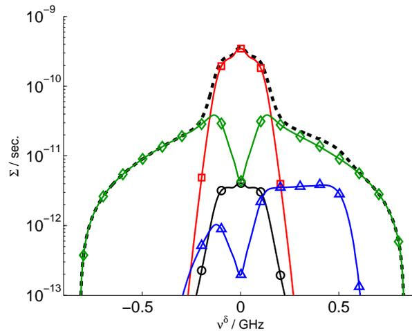
**Figure 12.** Scattering function for location in the NBI beam path; selection of near parallel velocities; scattering parameters:  $R = 6.18$  m,  $Z = 0.59$  m,  $\phi = 5^\circ$ ,  $\theta = 20^\circ$ ;  $\diamond$ -alphas,  $\triangle$ -beam ions,  $\square$ -bulk ions,  $\circ$ -electrons, ----total
