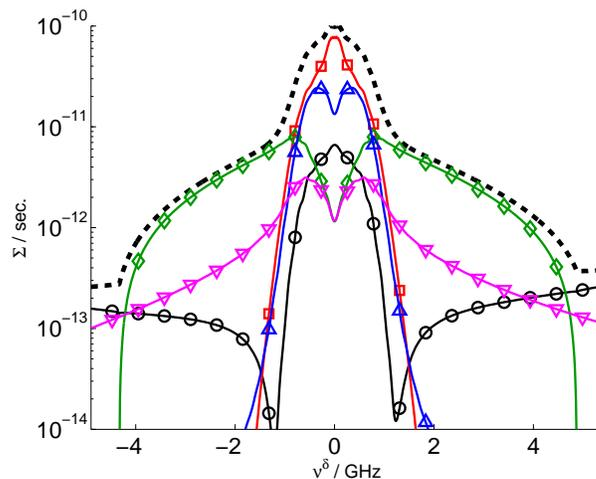
**Figure 7.** Scattering function for  ${}^3\text{He}$  minority heating with 2%  ${}^3\text{He}$ ; selection of near perpendicular velocities; scattering parameters:  $R = 6.76$  m,  $Z = 0.76$  m,  $\phi = 101^\circ$ ,  $\theta = 157^\circ$ ;  $\diamond$ -alphas,  $\triangle$ -tritons,  $\nabla$ - ${}^3\text{He}$ ,  $\square$ -bulk ions,  $\circ$ -electrons, ---total
