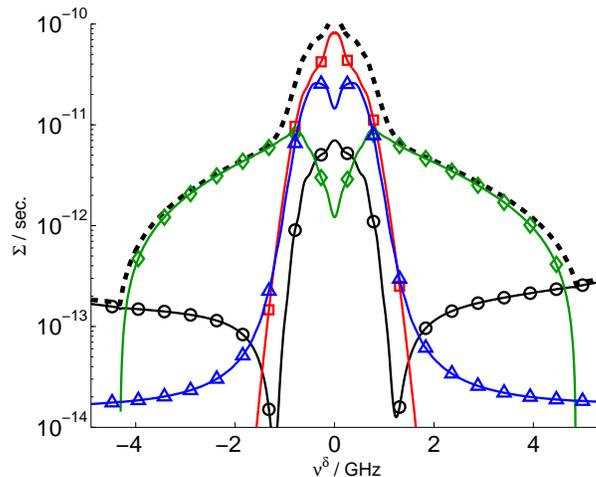
**Figure 6.** Scattering function for pure second harmonic tritium heating; selection of near perpendicular velocities; scattering parameters:  $R = 6.85$  m,  $Z = 0.77$  m,  $\phi = 101^\circ$ ,  $\theta = 156^\circ$ ;  $\diamond$ -alphas,  $\triangle$ -tritons,  $\square$ -bulk ions,  $\circ$ -electrons, ----total
