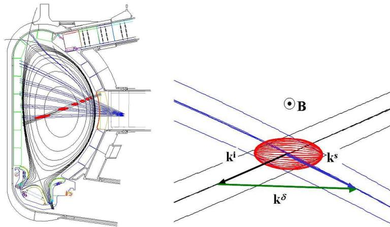
(a) One probe beam (b) LFS scattering geometry containing several the probe beam with wavenumber  $\mathbf{k}^i$  receiver beams (blue) in (black) and a receiver beam with ITER poloidal plane wavenumber  $\mathbf{k}^s$  (blue)
