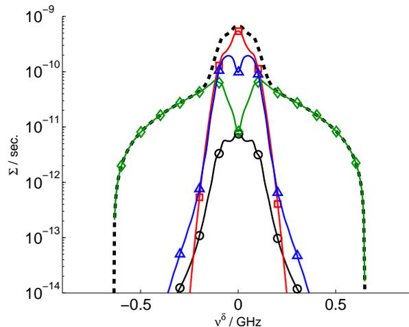
**Figure 10.** Scattering function for pure second harmonic tritium ICRH; selection of near parallel velocities; scattering parameters:  $R = 6.86$  m,  $Z = 0.59$  m,  $\phi = 2^\circ$ ,  $\theta = 16^\circ$ ;  $\diamond$ -alphas,  $\triangle$ -tritons,  $\square$ -bulk ions,  $\circ$ -electrons, ----total
