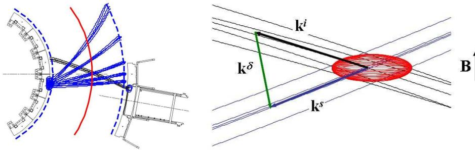
(a) One probe beam (black) crossing several receiver beams (blue) in ITER toroidal plane (b) HFS scattering geometry containing the probe beam with wavenumber  $\mathbf{k}^i$  (black) and a receiver beam with wavenumber  $\mathbf{k}^s$  (blue)
