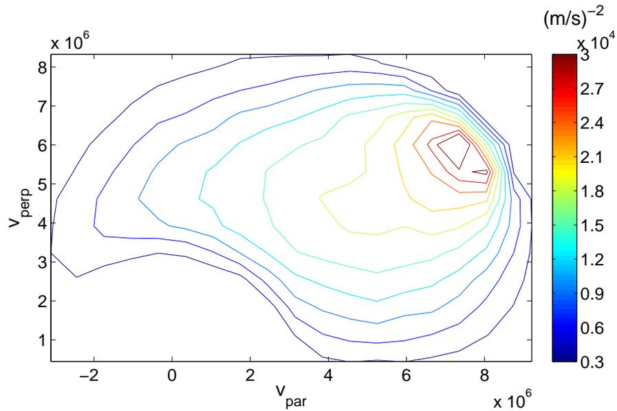
**Figure 4.** Beam ion distribution function for  $R = 6.12$  m and  $Z = 0.64$  m; isolines are equally spaced with a difference of  $0.3 \text{ (m/s)}^{-2}$  as indicated in the legend; the corresponding CTS signal is shown in Figure 9
