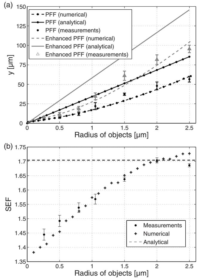
FIG. 3. (a) Distance between the bead position in the broadening segment and the channel wall  $y_{\text{PFF}}$  and  $y_{\text{EPFF}}$  in the PFF and EPFF device, respectively, as a function of the particle radius. Each measurement data point represents  $>300$  beads, and the error bars represents the standard deviation of the measurements. (b) The SEF as a function of the particle radius.
