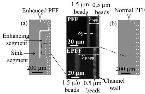
FIG. 2. Separation of polystyrene microspheres with radii of 0.5 and 1.5  $\mu\text{m}$  in (a) a PFF device and (b) an EPFF device. Each bead size is displaced further from the wall and the separation is amplified in EPFF with regard to the PFF device.
