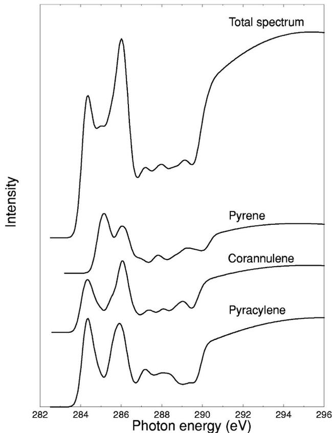
FIG. 4. Calculated NEXAFS spectrum with the individual components for the three different types of carbon atoms in  $C_{2v}$ - $C_{78}$ . These components are obtained by summing the individual spectra of the independent carbon atoms according to the pyracylene, corannulene, pyrene classification and scaling by their relative abundance.
