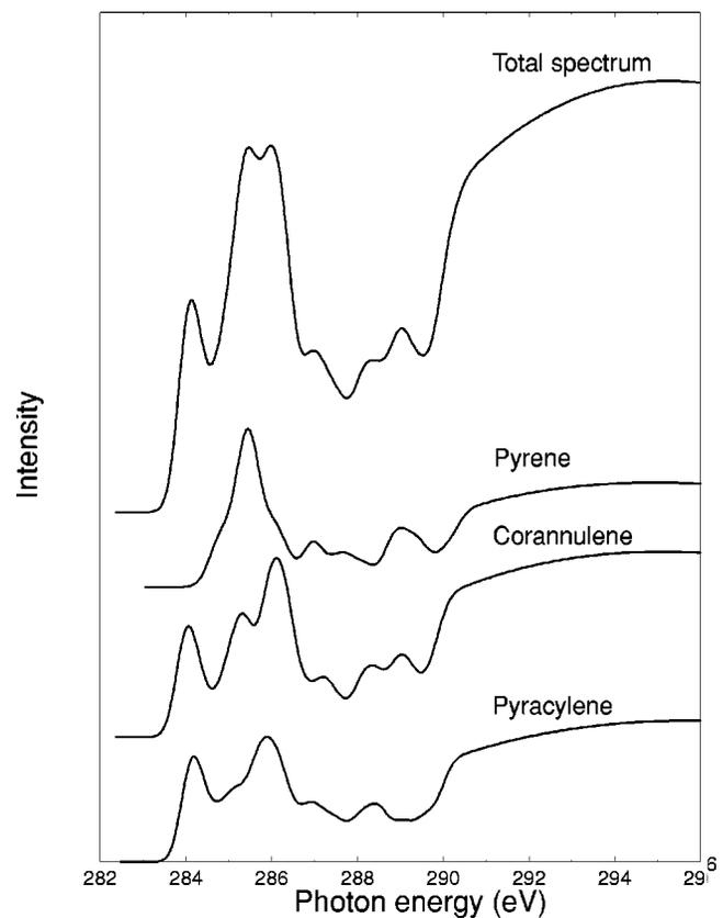
FIG. 5. Calculated NEXAFS spectrum with the individual components for the three different types of carbon atoms in  $C_{2v}'$ - $C_{78}$ . These components are obtained by summing the individual spectra of the independent carbon atoms according to the classification in pyracylene, corannulene, pyrene sites and scaling by their relative abundance.
