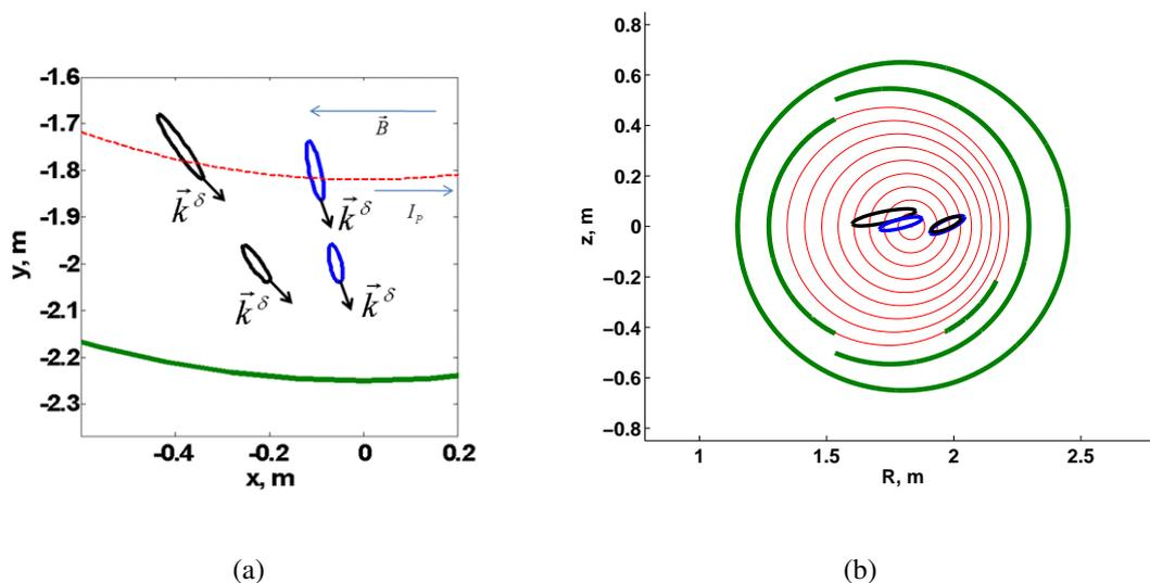
Figure 1: Geometry of the experiments. (a) Top view showing the plasma center (red) and the LFS limiter (green); (b) Poloidal view showing estimated flux surfaces (red) and limiters and the vacuum vessel (both in green). The blue and black ellipsoids in both figures denote the measurement volumes, where black corresponds to  $\phi \approx 140^\circ$  and blue to  $\phi \approx 110^\circ$
