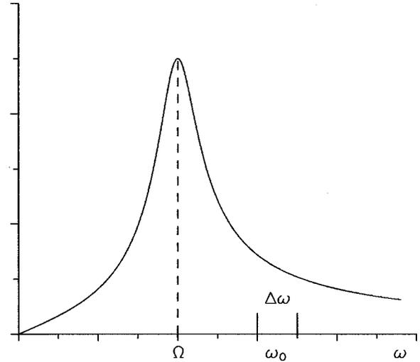
FIG. 3. Schematic (in arbitrary units) illustrating the essential elements of a cavity-induced synchronization mechanism: a sharp cavity resonance (peaked at  $\Omega$ ) and an off-resonance distribution of oscillator frequencies (center  $\omega_0$ , width  $\Delta\omega$ ).
